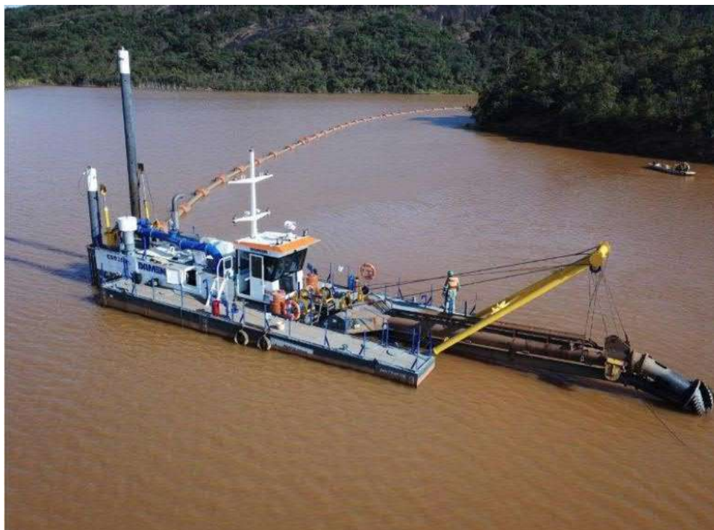
Figura 6-21: Cutter Suction Dredge - CSD
